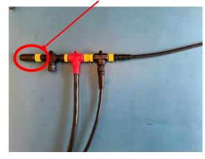
5. Plug in the NMEA Cable into the open port of the T-Connector you just installed. Make sure all of the cables and connectors are <u>screwed and secured tightly</u>.
